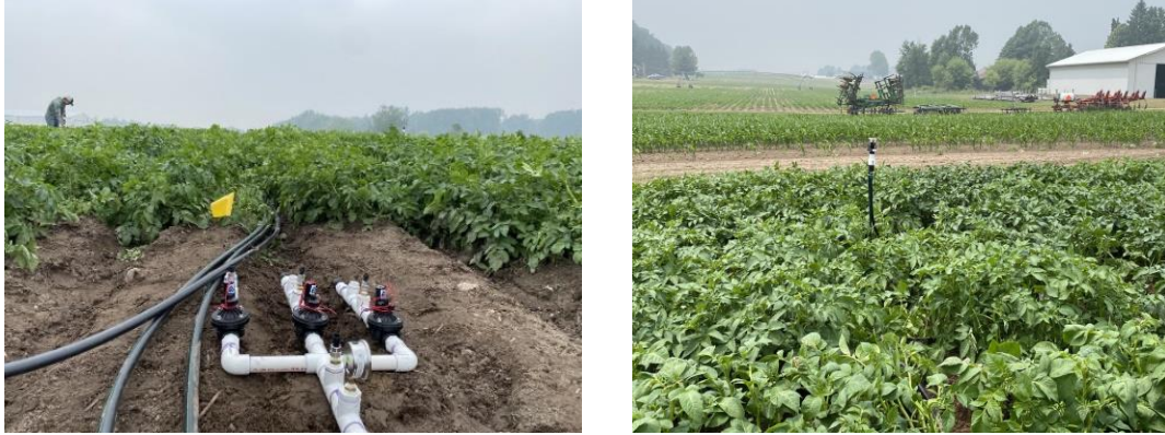
Figure 1. Installed Irrigation system, controlled by solenoid valves (Left). Xcel-Wobblers sprinklers by Senninger were used in this study (Right).
